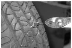
Inspect patched area! If the buffed area extends beyond the patch, look for any signs of tire casing body (ply) cords. Do not continue the repair if the buffed area exposes the tire's casing body (ply) cords; the tire must be scrapped.
